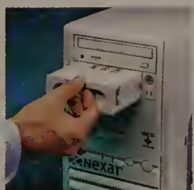
The hard drive carriage slides in and out on rails.
